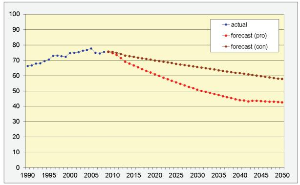
Figure 20: Transport power consumption in TWh.
