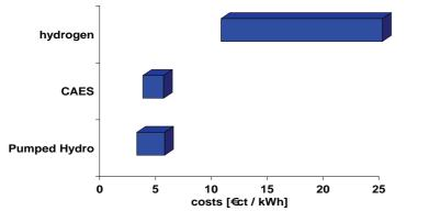
Figure 72: Comparison of storage systems for load-levelling (class B)
