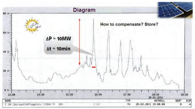
Figure 54: This is contrasted by a diurnal cycle of a photovoltaic area system with a power of 21 MV on a day with medium sky cover Quelle: Behnke, E.ON edis AG
