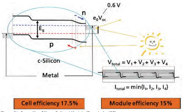
Figure 51: Crystalline Silicon Cell and Module (Fraunhofer ISE)
