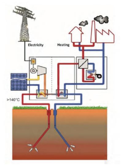
Figure 45: Geothermal Power Plant (Heinze et al. (2003)
