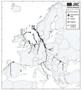
Figure 32: CO2 pipeline network in 2050, assuming joint international optimization. Total amount of CO2 captured and stored: 1145 Mt/y. (Ref: Fig 5.1 of [Morbee, 2012])
