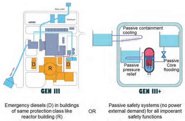
Figure 34: Passive systems applied in Gen III for the most important safety functions.
