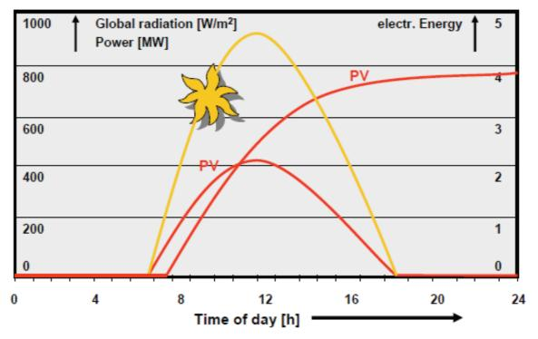
Figure 53: Solar energy-, power- and global radiation diagram on an ideal day
