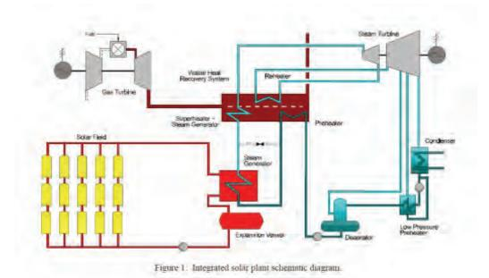
Figure 61: Example of a hybrid concept, the combination of solar heat to heat up feedwater in a CCGT. This concept is referred to as Integrated Solar Combined Cycle (ISCC). [Kelly et al., 2001]
