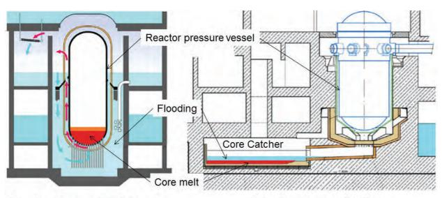
Retention of core melt in the reactor pressure vessel
