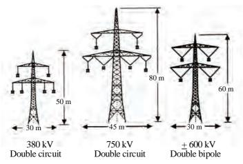
Figure 26: Tower images of AC and DC lines
