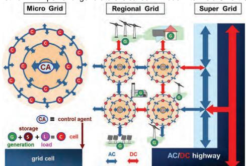
Figure 97: Structure of a future power supply system (Origin: Siemens)
