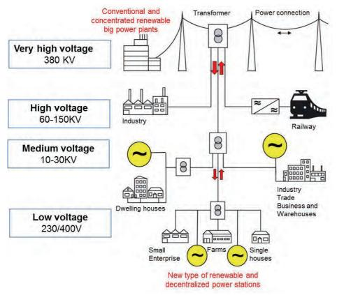
Figure 96: New structure of the power generation scheme
