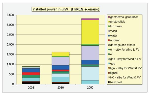
Figure 89: Installed power in GW in 2050 in EU27+ (HiREN scenario)
