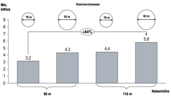
Figure 38: Additional generation of a 2 MW wind plant in South Germany due to the increase of the hub height and rotor diameter [IWES 2011]
