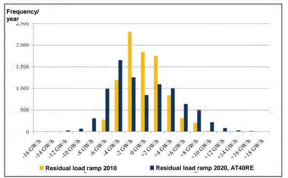
Figure 81: Gradients of the residual load changes over 1 hour, comparison of the year 2010 and 2020: scenario with 40% share of renewables in the generation mix, [VDE 2012]
