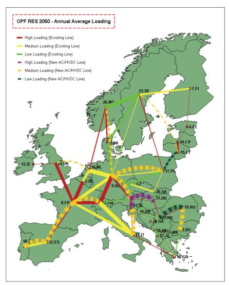
Figure 29: Annual Average Line Loading in 2050 (HVDC Expansion)
