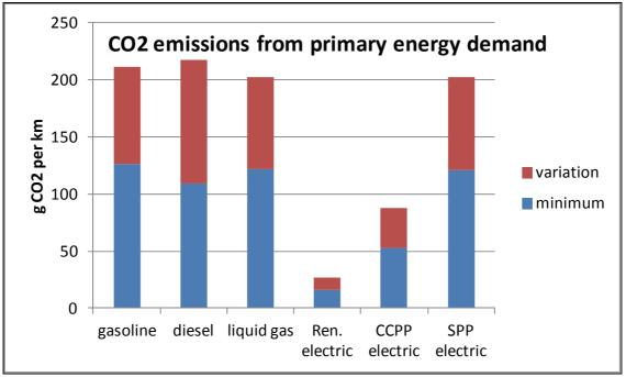
Figure 13: Specific CO2-emissions of power train concepts
