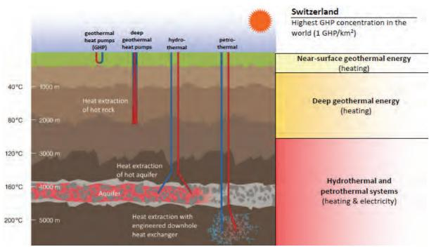
Figure 44: Geothermal energy use
